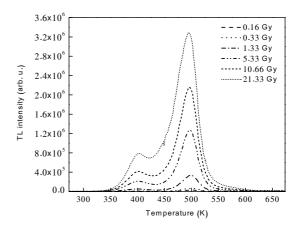
**Figure 1** Thermoluminescence glow curves of pellet-shaped sintered NaF:Eu<sup>3+</sup> samples after being exposed to  $\beta$  particle irradiation in the dose range from 0.16 to 21.33 Gy.
