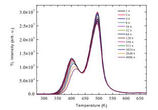
**Figure 3** Thermoluminescence glow curves of 2.6 Gy beta irradiated NaF: $Eu^{3+}$ , obtained after different elapsed time intervals between irradiation and the corresponding thermoluminescence readout.
