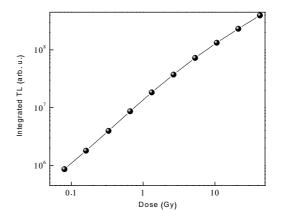
**Figure 2** Integrated thermoluminescence as a function of dose, of NaF:Eu<sup>3+</sup> pellets, exposed to  $\beta$  particle irradiation in the 0.08-42.0 Gy dose range.
